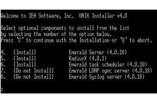
Once the system files have been installed, you are ready for the initial configuration of the Emerald Management Suite system. Installation сонрleted successfully. Systeн libraries have been installed in /usr/lib and /usr/local/iea Database configuration file has been installed to /usr/local/iea/odbc.ini
